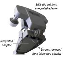
4. Slide the LNB into the integrated adapter, and re-install the two screws (removed earlier) through the integrated adapter and LNB.
